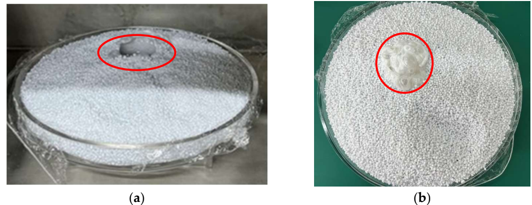
Figure 16. PET melting regions are marked by red circles. (a) # 9 * in Table 1 when the maximum temperature is 196 °C. (b) # 2 * in Table 1 when the maximum temperature is 220 °C.
